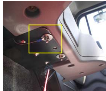
Mount the ground wire to metal surface.
