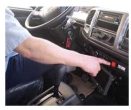
The HTS uses a dash release button with a flashing light and audible alarm to warn the driver if the hand truck is not locked in the Ultra-Rack. Also has a manual key override on the Ultra-Rack frame.
